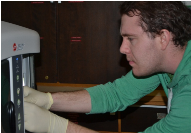
Kurt Simmons loading a sample for analysis using a Beckman Coulter Multisizer. This technique provides size distribution and quantification of particulates in a water sample, allowing for changes in particulate concentrations to be tracked as sea cucumbers feed (photo credit: Jeff Clements).
